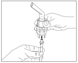
Connect the other end of the hose [6] to the hose connector [4] on the nebuliser by lightly turning it.
