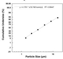
Measurements were performed using a sodium fluoride solution with a "Next Generation Impactor" (NGI).
